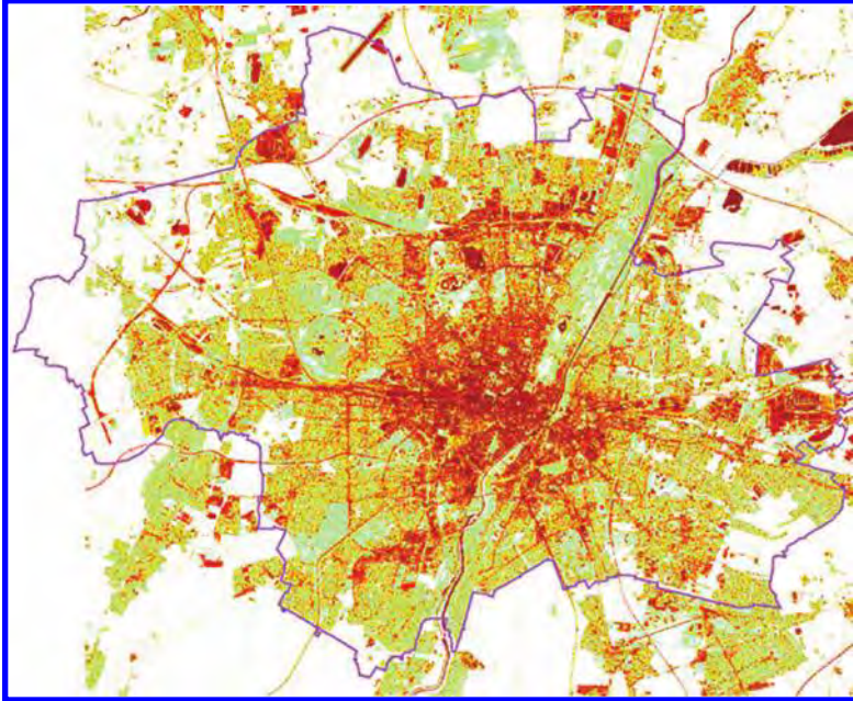
COLOR FIGURE 11.9 Pixel-based soil sealing map of Munich, Germany. (Courtesy of GSE Land – H.G. Geodata Solutions.)
