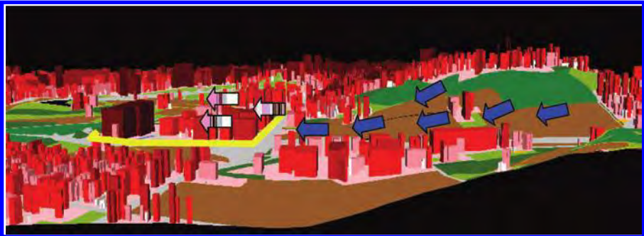
COLOR FIGURE 15.3 Perspective view of a section of Osnabrueck: newly constructed buildings (yellow outline) block the flow of cold and fresh air toward the center of the city showing the impact that such a structure would have on the inner-city environment (exaggeration factor 5).
